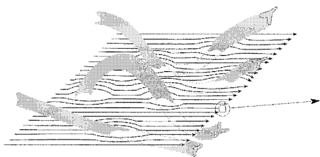
Fig. 19: Laminar flow of smoke gases in the filter. The flow curves always run around the acetate filaments.
